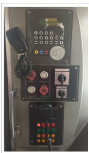
Figure 3. The in-train PA communication panel in the driver's cabin. Source: Author's personal collection.
