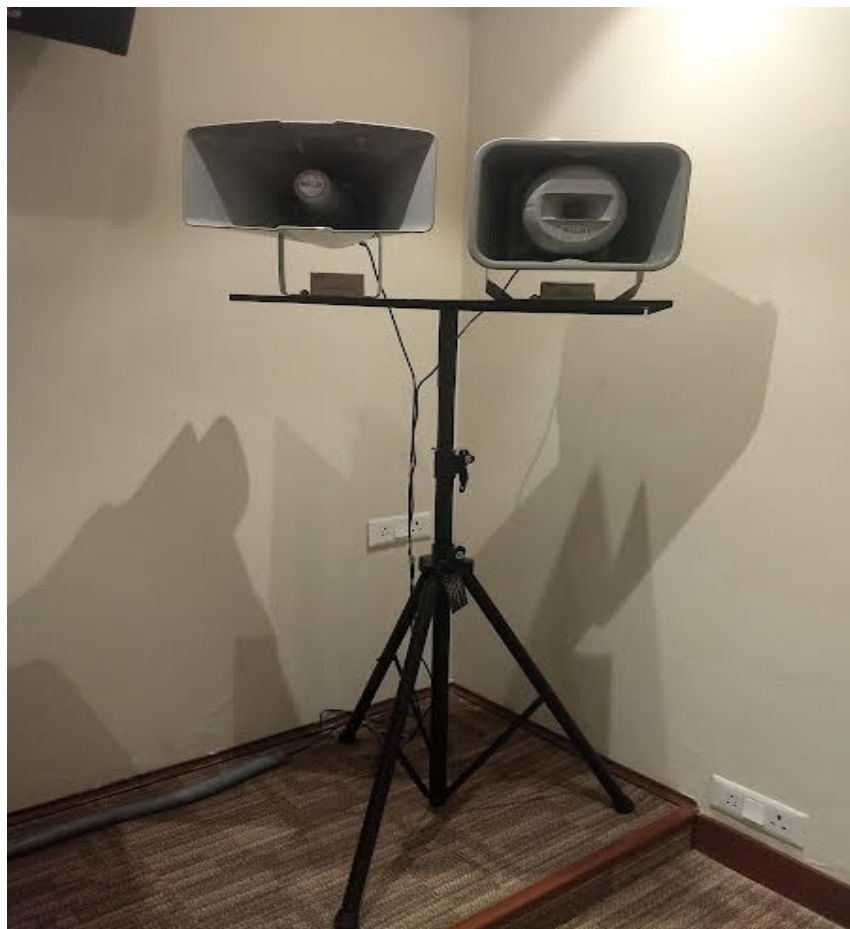
Figure 5.6: Two kinds of horn speakers (the one to the left is used in factory spaces, and the one to the right is a music horn and is used in temples). Source: Author's Personal Collection
